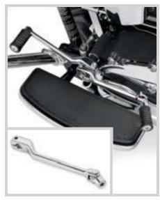
A. FOLDING HEEL SHIFTER – RETRACTED POSITION
