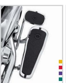
I. TAPERED RIDER FOOTBOARD KIT WITH CRESTED BAR & SHIELD LOGO INSERT (SHOWN WITH BRAKE PEDAL PAD)
