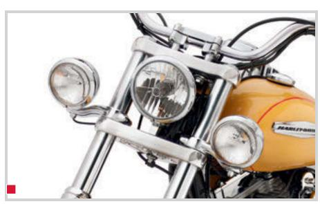
A. AUXILIARY LIGHTING KIT – 68605-08A SHOWN (SHOWN WITH AUXILIARY LAMP BULB KIT)
