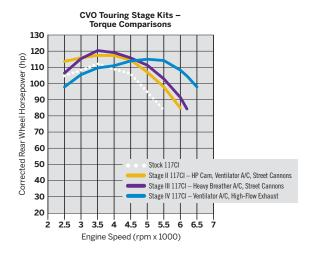
DYNAMOMETER (DYNO) PERFORMANCE TESTING: Declared performance values in this catalog represent SAE J-1349 transient peak power output.
