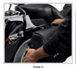
Slide the bag rearward to disengage the mounting bracket and lift the bags away.
