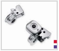
B. CHROME CLUTCH BRACKET AND MASTER CYLINDER KIT – (45355-08 SHOWN)
