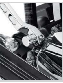
**B. HEEL/TOE SHIFTER SHAFT COVER**
