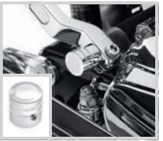
D. HEEL/TOE SHIFTER SHAFT COVER
