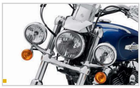
A. AUXILIARY LIGHTING KIT – 68000110 SHOWN (SHOWN WITH TURN SIGNAL RELOCATION KIT AND AUXILIARY LAMP BULB KIT)
