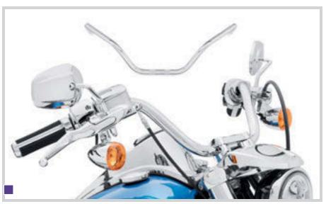
\*NOTE: Installation of some handlebars and risers may require a change in clutch and/or throttle cable and brake lines for some models. Handlebar height is regulated in many areas. Check local laws before installation.
